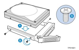
Figure 18. Attaching a Hot-swap Hard Disk Drive to a Carrier
